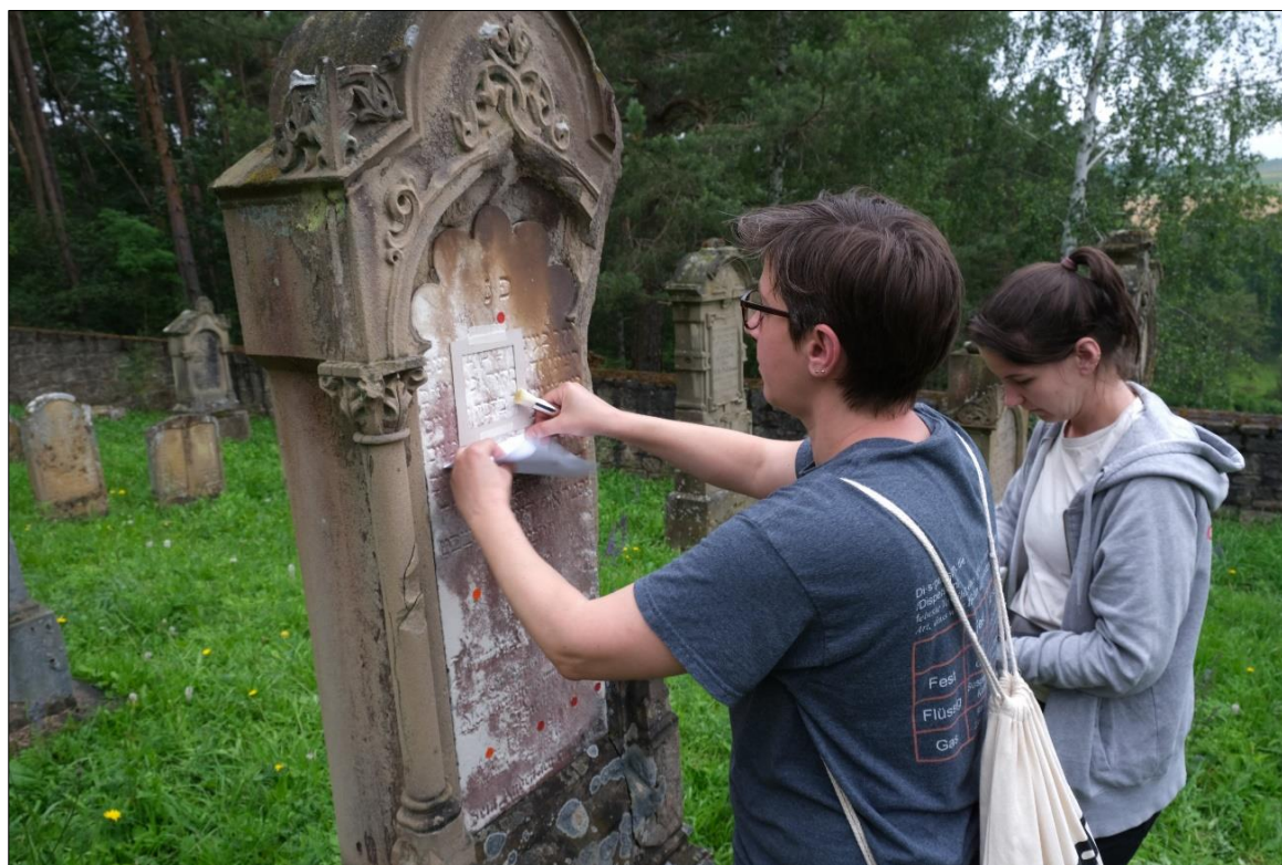
Fig. 11: Implementation of the “Brush test” for the evaluation of the superficial material loss and decohesion
